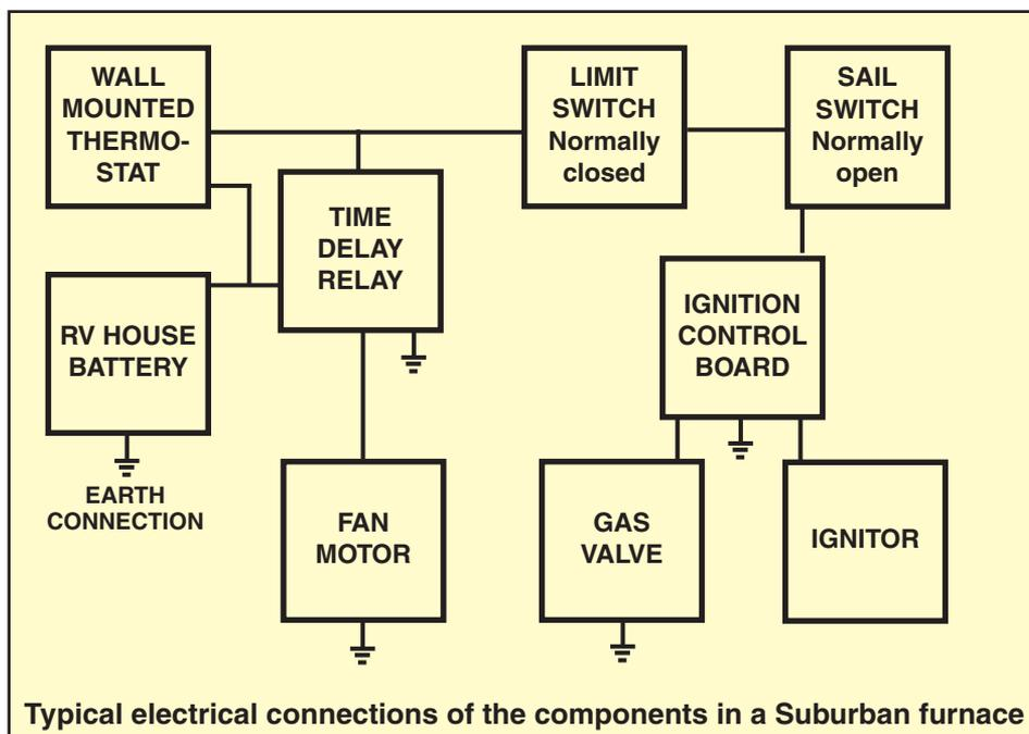
**Typical electrical connections of the components in a Suburban furnace**
