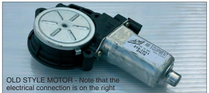
OLD STYLE MOTOR - Note that the electrical connection is on the right
